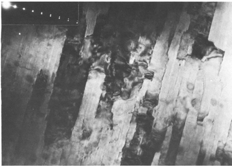
Figure 1 Low-angle [hk.0] tilt boundaries in sodium beta alumina. The tilt boundaries are normal to [00.1] .
